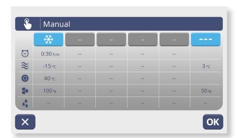
The VINTOS as well as the VINTOS+ offer the possibility, to manually generate customized programs for a specific cycle. The input is simple and allows for an individual setting of time, temperature and fan speed.
